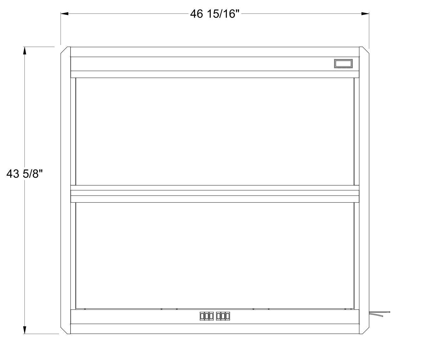
Electrical Requirements: 120VAC, 60 Hertz, Single Phase Power Rating: 7.2A Rough Opening Dimensions: 41 1/4" x 44 11/16"
