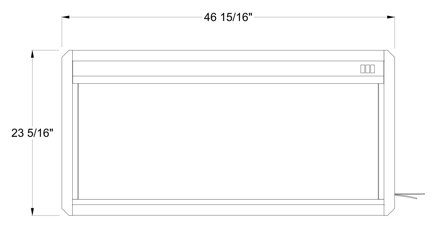
Electrical Requirements: 120VAC, 60 Hertz, Single Phase Power Rating: 3.6A Rough Opening Dimensions: 21" x 44 11/16"
